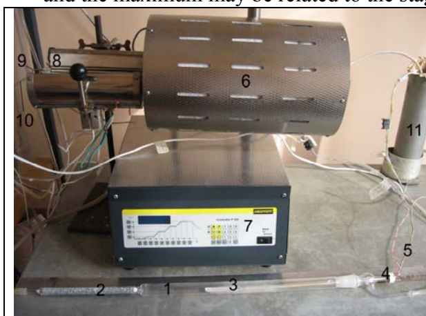
Fig. 1 (on the left side). Disassembled view of the setup for the tritium release experiments: 1 and 2 – compartments of the quartz tube for the sample and for a bed of granulated zinc respectively; 3 – a porcelain boat for the sample under study; 4 – a white cylindrical ceramic holder for the cold junction of a type S thermocouple of 300 mm in length; 5 – a type K thermocouple to measure the temperature of the cold junction of the type S thermocouple; 6 – a “Nabertherm” RT 50-250/13 tube furnace; 7 – a P 320 controller for the “Nabertherm” tube furnace; 8 – a tube furnace for heating the zinc bed; 9 and 10 – measuring and driving type K thermocouples for the zinc bed respectively; 11 – an ice bath for the cold junctions of type K thermocouples 5 and 9.
